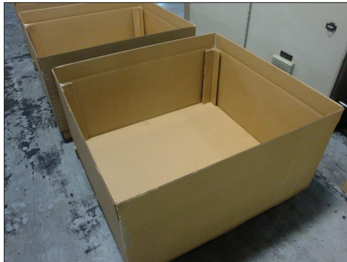
Figure 5.3.10: Example of Corrugate Corner
