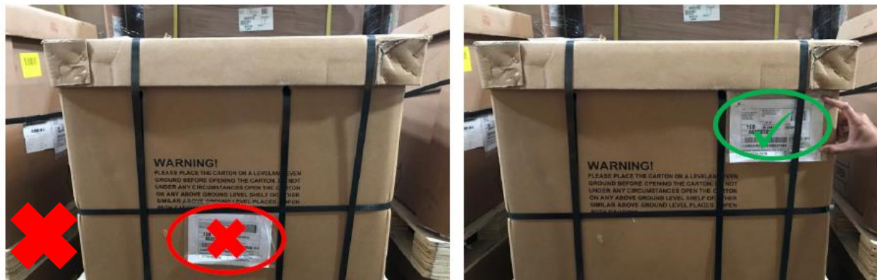
Figure 7.0.3.2: 1724 Label Location Non-Compliant vs Compliant
