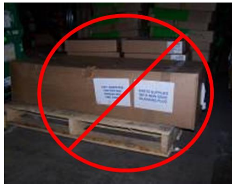
Figure 5.3.4: UNACCEPTABLE- Cartons are NOT to extend over the edge of the pallet
